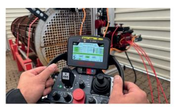
Everything under control: the cleaning process is controlled by a joystick
